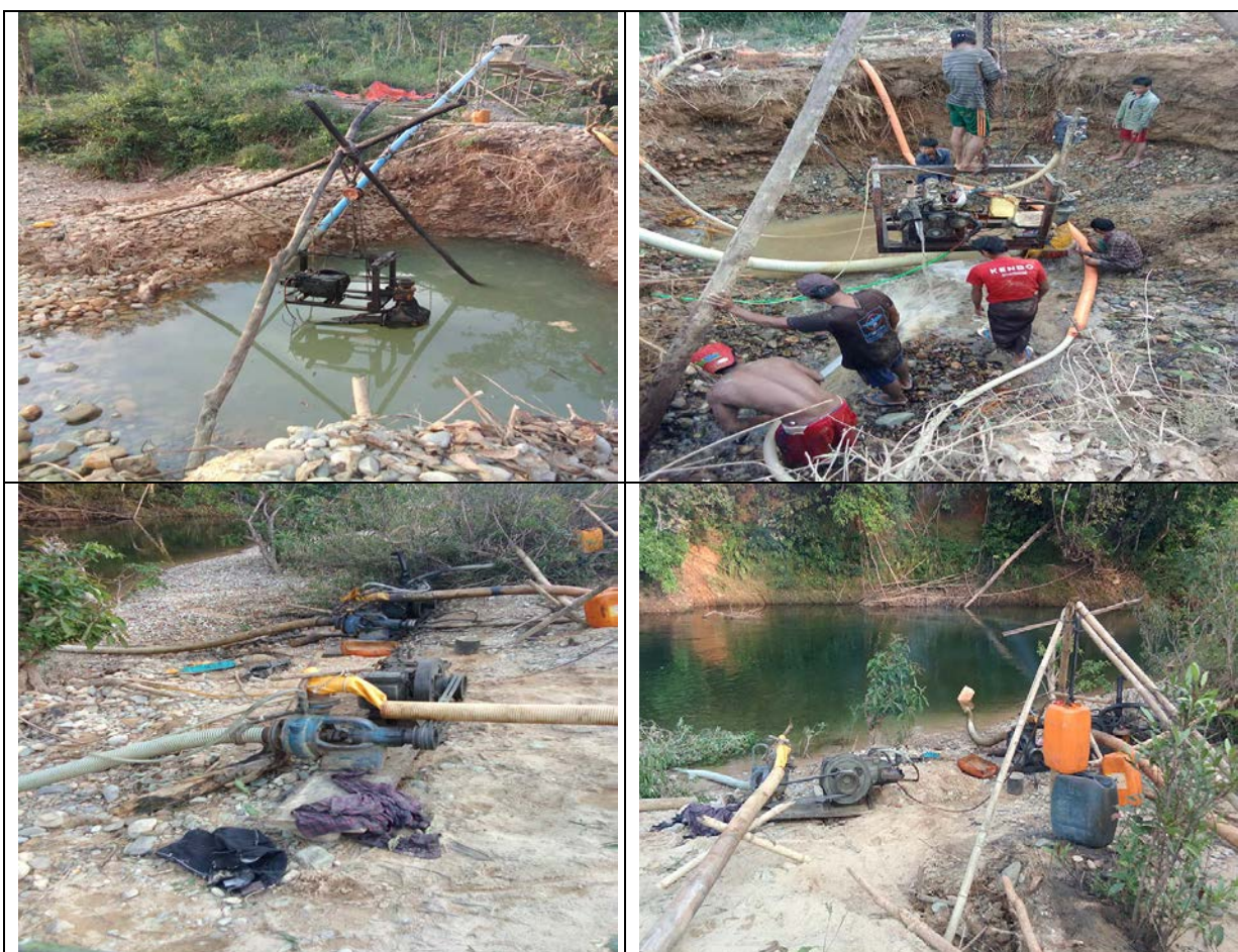
These photos were taken on January 12 th 2018 in Htoo Maw village, La Baw sub-area, Kleh Muh Htee main area, K'Ser Doh Township, Mergui-Tavoy District. The photos on the top row show the process of lead mining. The photos on the bottom row show how the lead was mined near a stream. The machine pumps water from the stream and transfers it to the lead mine. It returns the water to the stream, contaminating a local water source. [Photos: KHRG]
